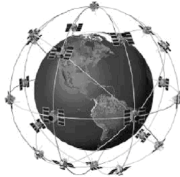
21 activated satellites are continuously sending unique signals while surrounding the Earth
