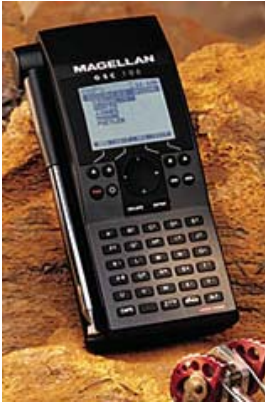
A handheld GPS can measure and log positions on Earth by triangulating the position of satellites
